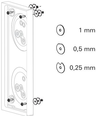
8. Pass the connection cable completely through the installation box and housing openings, insert the housing into the installation box and tighten the mounting screws (but not so tight that the housing cannot be moved).
