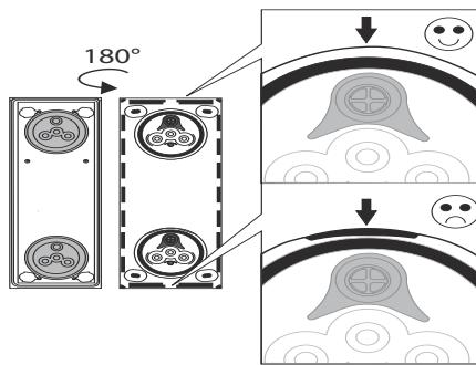
9. Insert the modules into the function carrier (observe TOP mark) and lock them in place. For detailed information about the modules, see the operating instructions for the individual modules.
