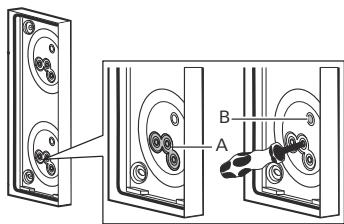
7. Insert the mounting screws of the mounting corners through the openings of the housing.
