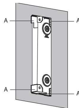
3. Do not apply any pressure to the adhesive bond for at least 15 minutes. The final strength of the bond is reached after 72 hours.
