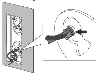
Cut the connection cable to length and connect it to the plug terminal (A). Turn the plug terminal by 180° (B) and plug it into the connection on the voice or door station module.
