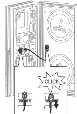
12. Using the locking key, slightly tighten the screw for locking the housing (0.6 Nm) at an angle of 90°.
