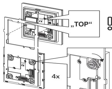
10. Pivot the function carrier into the housing (A). When installing 3- to 5-gang housings, pay attention to the additional catch mechanism (B).
