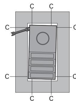
14. Disengage the function carrier, loosen the safety bond and put the function carrier plus modules to one side.
