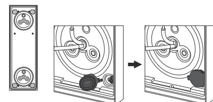
17. Connect the terminating resistors to the function carrier with the modules, followed by the system cable. Always connect a terminating resistor to the first and last modules on the system cable. Observe the plug coding!
