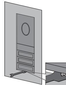
13. Use the locking key to adjust the installation box positioning screws (C) so that the gap between modules and the front plate is symmetrical. Then tighten all positioning screws.
