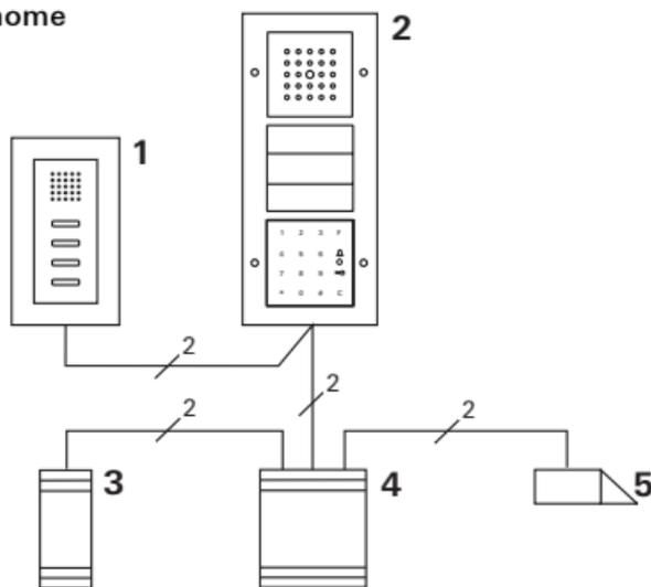
The keypad can be connected to the Gira flush-mounted door stations and to the built-in loudspeaker. The keypad can control up to 16 switching actuators (8 group actuators + 8 individual switching actuators) and the door opener function. In addition, home stations can be called directly from the door communication system.
