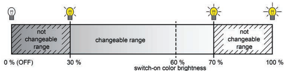
Figure 30: Example of a brightness range with switch-on brightness
