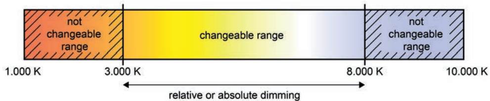
Figure 36: Example of a dimmable colour temperature range
