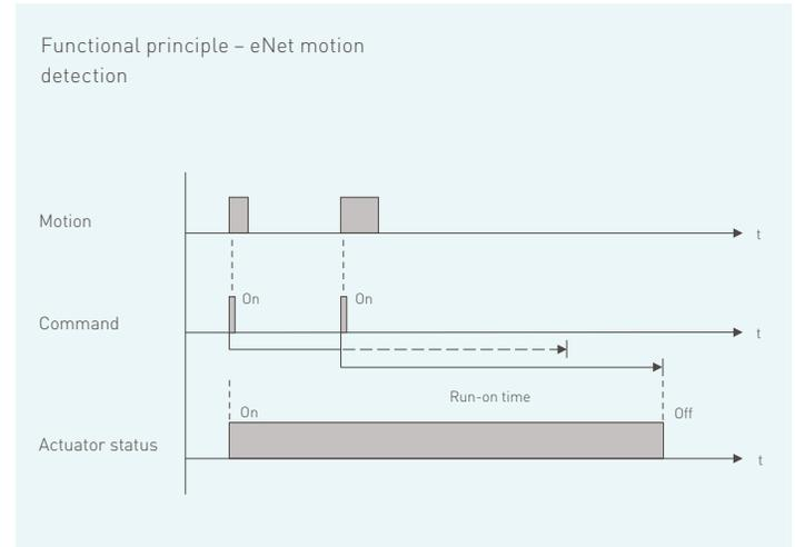
the run-on time has elapsed, the actuators automatically switch their loads back off again. If an actuator receives commands with different run-on times from several connected motion detectors, the longest run-on time always applies.
