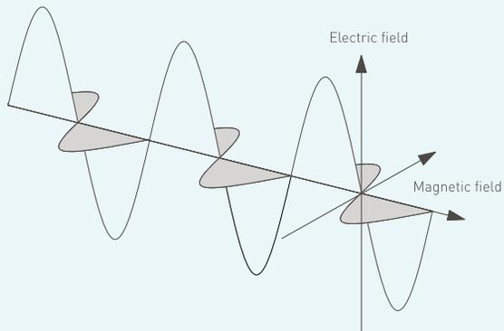
Radio waves with a low to medium frequency do not have enough energy to stimulate matter, but can penetrate building ceilings or walls. Depending on the mass (thickness) and conductivity (metal content, moisture), this is associated with high energy loss to a greater or lesser extent.
