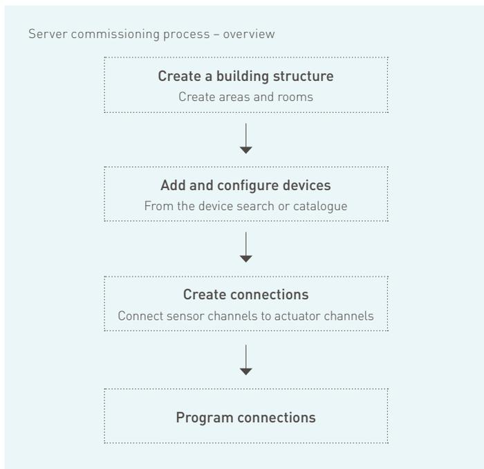
The devices are then assigned to the room they were installed in (device location). The individual device channels are each assigned to the room they “have an effect on” (channel location). The channel location is shown in the app later on. The device location of a 4-gang DRA switching actuator may, for example, be “Cellar”, while its actuator channels may be assigned to the living room, bedroom, working room and bathroom channel locations.
