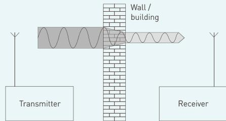
Caution is advised if a building is equipped with shielding materials to reduce "electro smog". Flush-mounted boxes with conductive coatings are hardly suitable for wireless products; special
