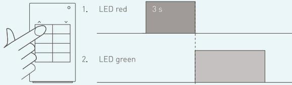
Transmission successful, all actuators switched off or all shading solutions are in the resting position (0 %, shading solutions retracted)
