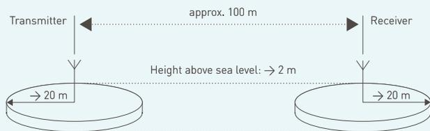
“free field”, in which range measurements are performed too. The free field and the free space differ in that, in the free field, some of the radio waves are reflected on the ground and overlap with the directly radiated wave.
