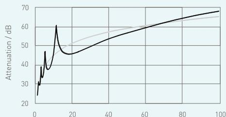
spherical shape. In the far field – at 868 MHz from approx. 2 m – the radiation power arriving at the receiver drops to the square as the distance increases. The attenuation on the transmission path is specified in decibels [dB] in technical documentation.
