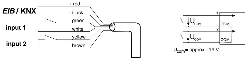
A spacing of 4 mm minimum between extra low-voltage lines (bus and extension inputs) and the load lines (230 V) must be ensured (see fig. A).
