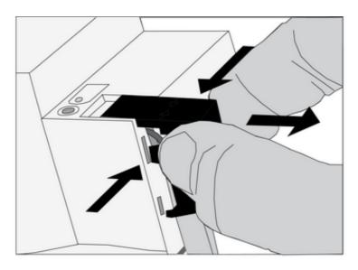
Figure 4: Removing the cover
