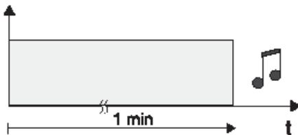
5. The programming mode ends automatically after about 1 minute or can be terminated by a short depression of the programming key. The radio-control pushbutton is then again in the normal operating mode.
