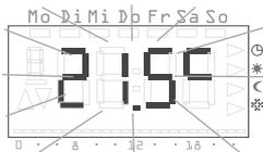
✓ The room temperature controller returns to the normal display and regulates the set individual temperature until the next switching time in the time program. As long as the individual temperature is used as the setpoint input, no operating mode (Comfort, Lowering, Anti-freeze) is displayed, since none of the temperatures stored there is valid.
